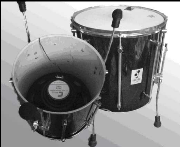
A Loudspeaker as Drumhead
